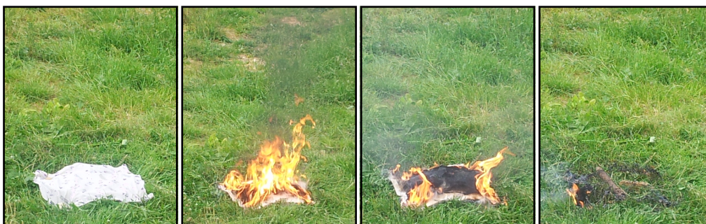
Figure 14: Burning of the gasoline fire in 4-picture time series. Fire size 50 × 50 cm.
