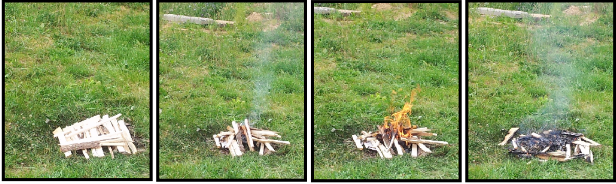
Figure 16: Burning of the wood cellulose fire in 4-picture time series. Fire size 50 \times 50 cm.
